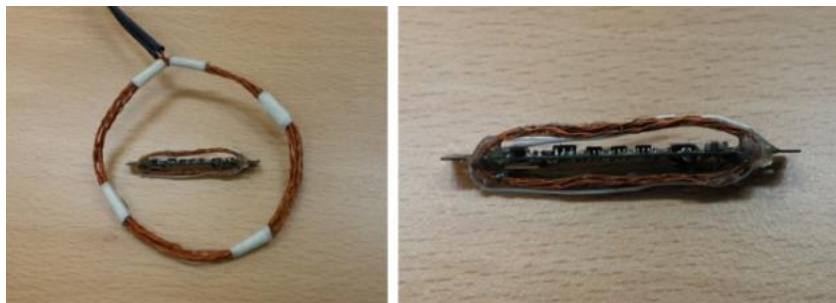
Figure 1. Round transmitting coil (Tx coil, left) and elliptical receiving coil (Rx coil, right).
