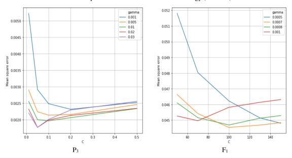
Figure 7: Plot of MSE for various Gamma and C values of SVR for 6 Soft Sensor Models
