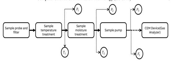
Figure 1: Block Diagram of Sample Handling System
