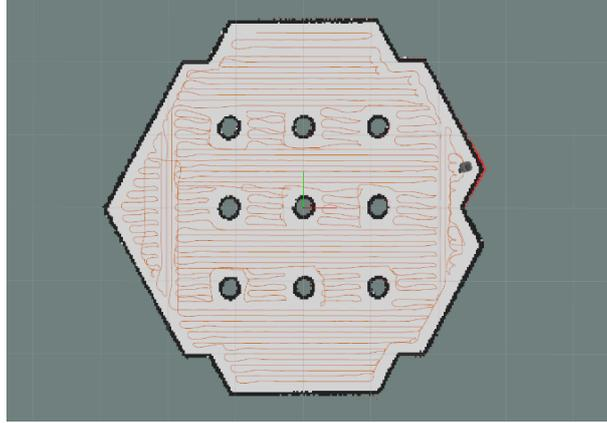
Figure 6: Robot trajectory during execution of generated path
