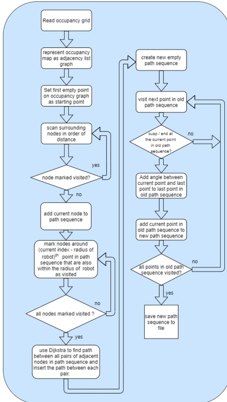
Figure 3: An Excerpt of the Path Generation and Cleaning Algorithm
