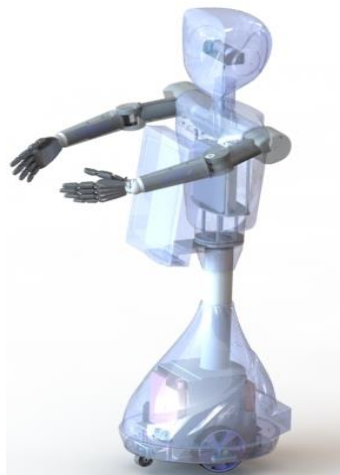
Figure 1. The mechanical structure of MiABot reception robot.
