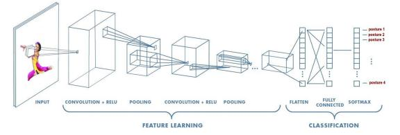
Figure 4. Neural network with many convolutional layers
