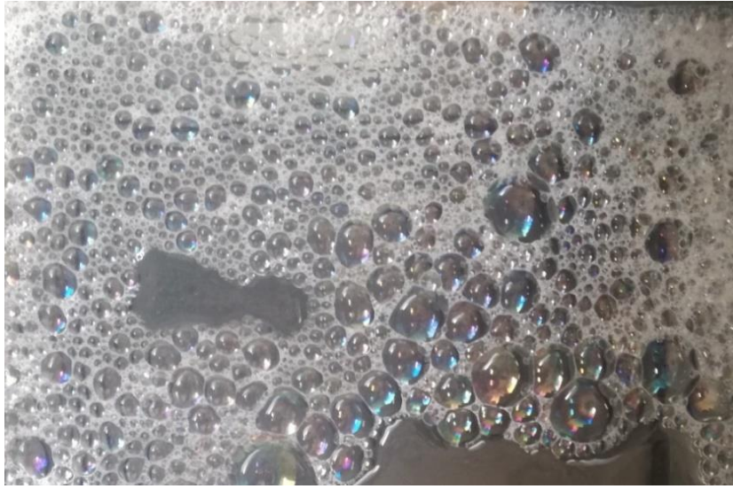
Figure 3. Bubbles accumulation after 4 minutes foaming at flow rate 100l/h and X_e=0.224
