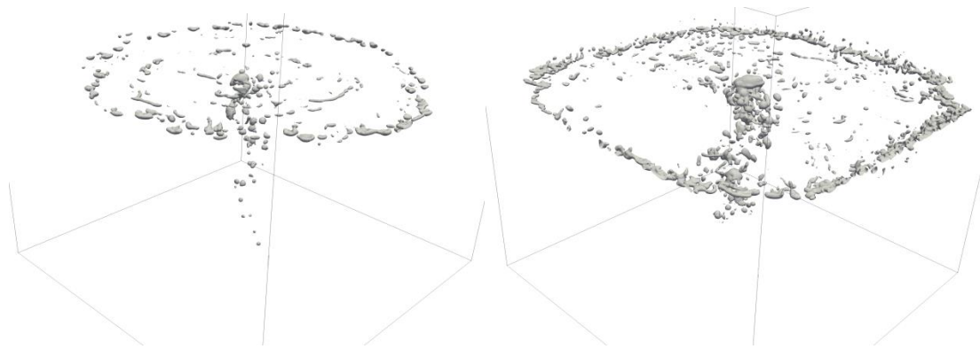
Figure 7. Bubble structures at the liquid free surface for periodic side vertical boundary (left) and wall type vertical boundary (right)
