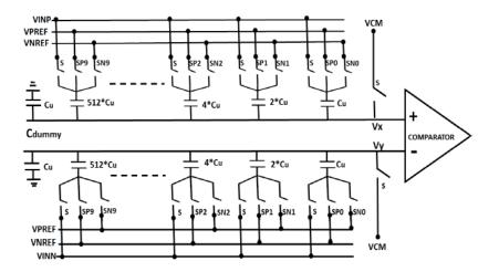
Figure 4. Architecture 10-bit fully differential CDAC
