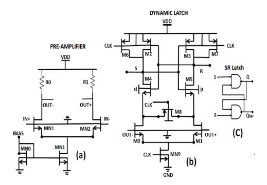
Figure 5. Schematic of preamplifier based dynamic latch
