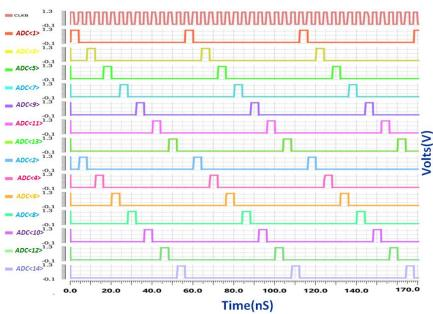
Figure 17. Transient response of timing scheme
