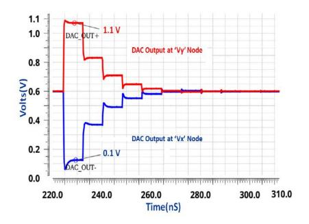
Figure 7. Transient response of 10-bit CDAC
