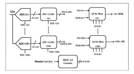
Figure 18. Block diagram of 14×1 digital multiplexing
