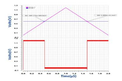
Figure 8. Transient response of dynamic comparator
