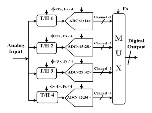
Figure 1. Architecture of 4-Channel TI-ADC.
