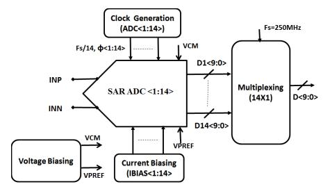
Figure 14. Block diagram of single channel 10 bit, TI-SAR
