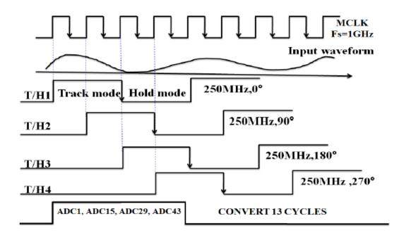
Figure 2. Timing diagram of 4-channel TI-ADC.
