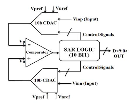
Figure 3. Block diagram of 10-bit SAR ADC
