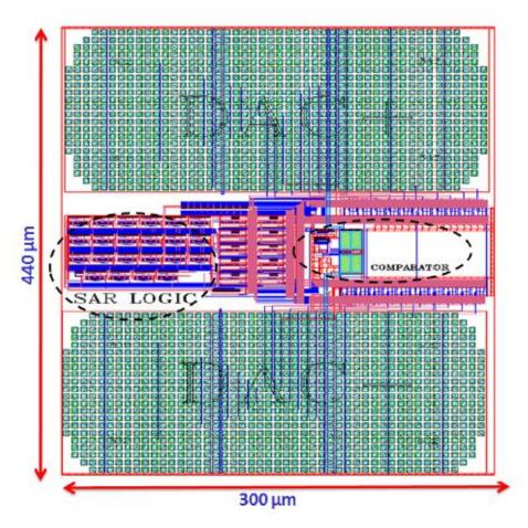
Figure 11. Layout of 10-bit SAR ADC
