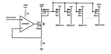
Figure 15. Schematic of voltage to current converter
