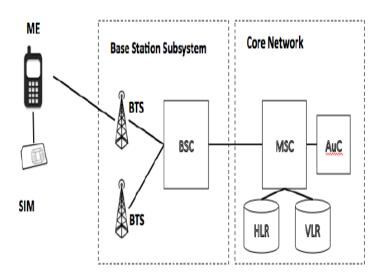
Figure 1. The basic structure of the GSM network
