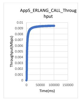
Figure 10. The throughput for GSM-FR
