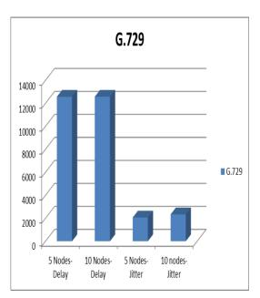
Figure 13. Variation in jitter and delay for G.729
