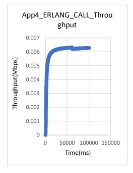
Figure 9. The throughput for G.723
