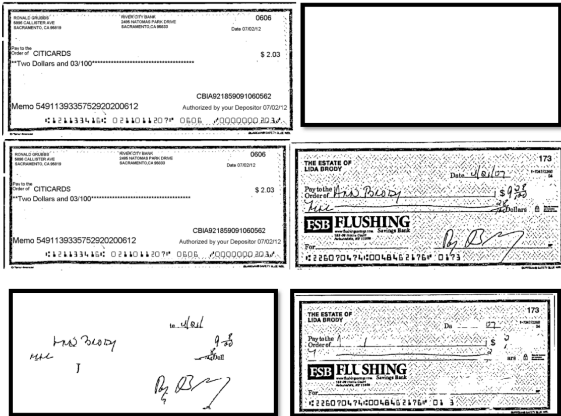
Fig 6. (a, b, c, d, e, f, raster order): a: a check without handwriting, b: the result of handwriting detection where nothing detected, c: the original check by ANDING, d: a noisy bank check, e: detected handwriting, f: original check by ANDING. (almost complete performance).
