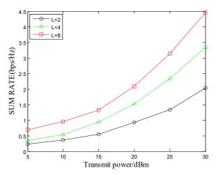
Figure 7 Diagram of sum rate with transmission power for different multipaths
