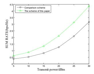
Figure 6 Diagram between sum rate and transmission power
