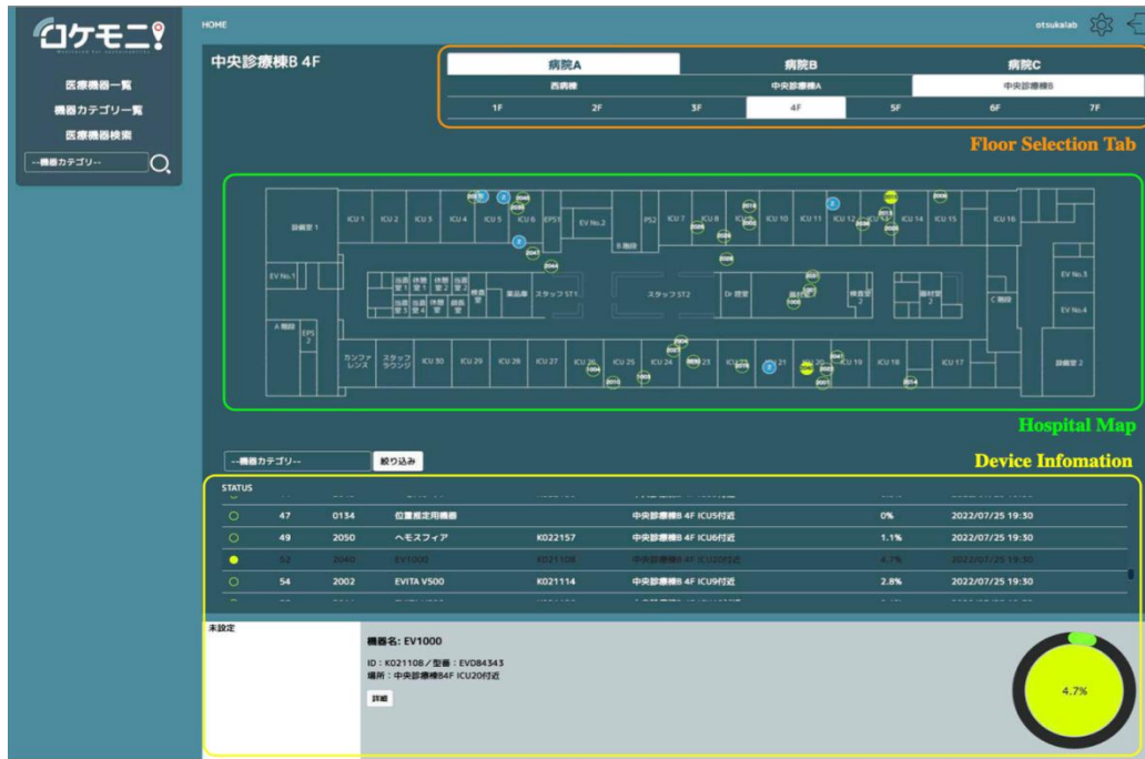
Figure 7. Visualization Web Page. Circle icons in the hospital map indicate the location of medical devices. The color of the icon indicates the status of the device.
