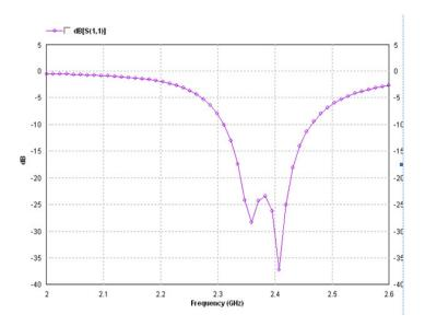
Figure 10 Reflection coefficient.
