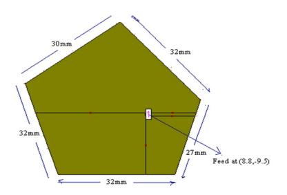
Figure 9 Geometry of the pentagonal patch.
