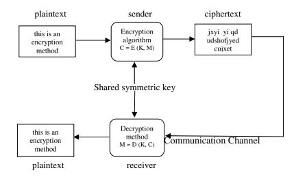
Fig 1: Symmetric encryption system
