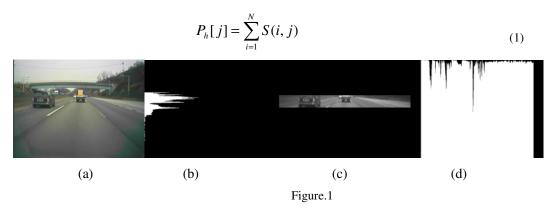
From the Fig.1 (b) horizontal edge profile, it is clear that upper most  $(U_p)$  and lower most peaks  $(L_p)$  corresponds to regions in which vehicles needs to be searched. Fig.1(c) shows the vehicle localized region. Also a vertical profile is constructed on the localized region obtained from horizontal edge profile. Vertical profile is the sum of vertical gradient pixel values perpendicular to the y axis and is represented by the vector  $P_y$  of size N columns and is defined by:
