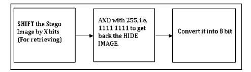
Fig. 2. Block diagram for extracting the hidden image
