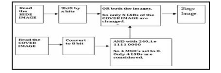
Fig. 1. Block diagram of LSB Steganography
