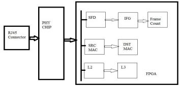
Fig: Block Diagram Of Ethernet Packet Processor
