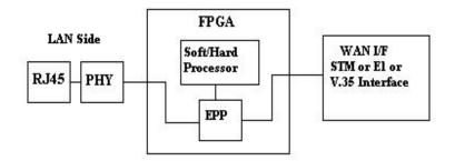
Note: EPP (Ethernet Packet Processor), PHY (10/100/100 Physical interface). RJ45: Ethernet Connector
