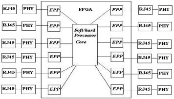
Note: EPP ( Ethernet Packet Processor), PHY ( 10/100/100 Physical interface). RJ45: Ethernet Connector
