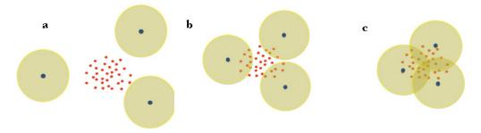
Figure 3. Three sensor placements scenarios: (a) none of the targets are observed by sensors and the, (b) a large portion of targets are missed due to lack of proper placement of the sensors, and (c) sensors are observing all targets and have a better placement compared to both cases (a) and (b). in this figure blue dot denotes the mobile robots carrying sensor(Limited Sensing Range (LSR) sensor), yellow bordered circle is the sensing range, and red dots are the targets.
