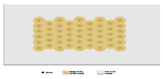
Figure 8. Case 4, when the number of sensors is too less than what is required to cover the region in which tracking is to be done.
