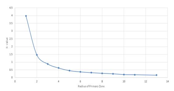
Figure 10. Comparisons of K-values v/s Radius of primary zone of the sensor.
