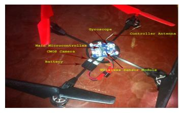
Figure 3. Structure of home-made quadcopters
