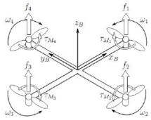
Figure 2. Whole structure of rotation of rotors in quadcopter
