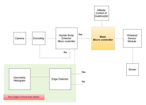
Figure 6. Block diagram of human detection in quadcopter
