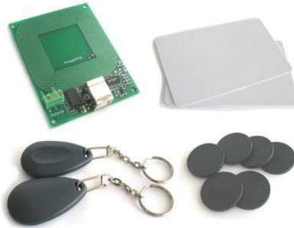
Fig. 3 Reader, cards and tags RFID
