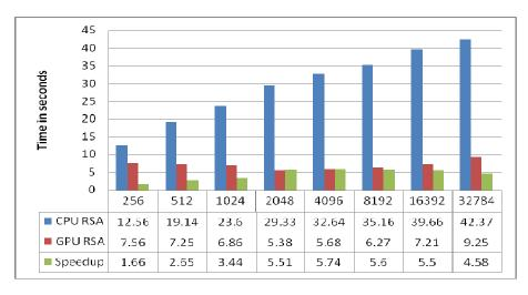
Figure 4. Graph showing effect of data input on CPU RSA and GPU RSA along with the Speedup
