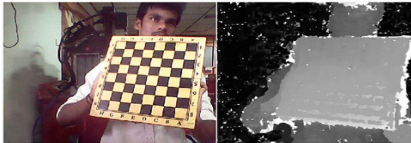
Figure 7: Image from the left camera (left), Computed disparity map (right)
