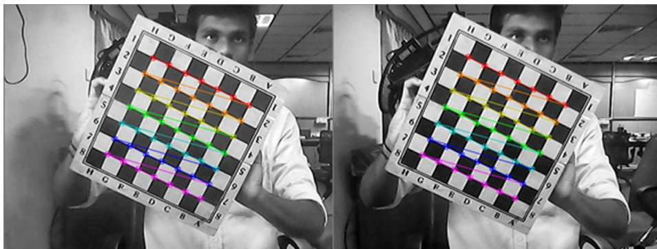
Figure 4. Stereo camera and rig calibration using chessboard as a calibrating object. Detected chessboard corners are marked in simultaneously taken left and right images.
