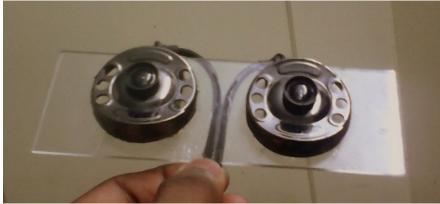
Figure 3. Stereo camera rig made from two webcams.
