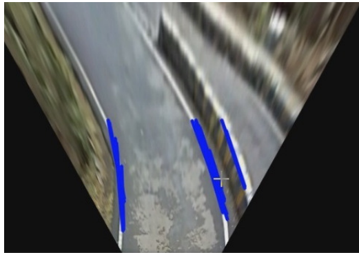
figure 4(a). Bird's eye view of detected curvy lanes using mean value theorem on centroids of Hough lines on curve without color thresholding. Noise filter and shadow/illumination correction is also applied here.
