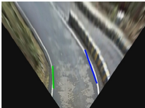
figure 5. Bird's eye view of result obtained from algorithm to differentiate various curves using slopes of tangents (from mean value theorem)
