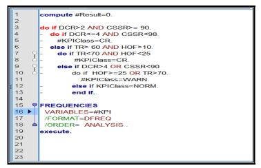
Figure 1. Fault classification algorithm
