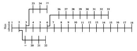
Fig. 2: Standard IEEE-33 bus test system
