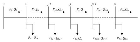
Fig. 1. Single line diagram of a radial feeder [8]
