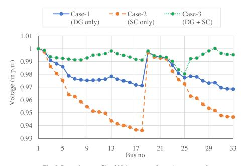
Fig. 5: Bus voltage profile of 33-bus system for various case studies
