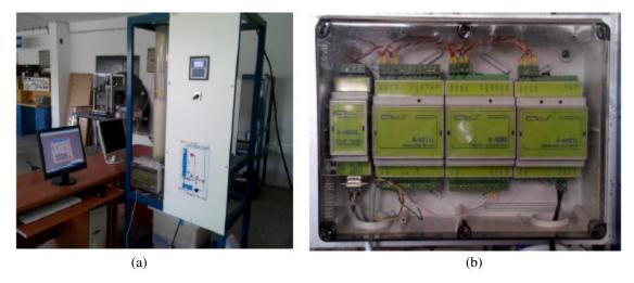
Figure 4. (a) The liquid level control system with computer-controlled and (b) DAQs
