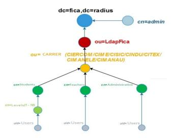
Figure 3. Hierarchical structure LDAP - FICA
