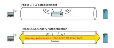
Figure 1. EAP-TTLS Method
