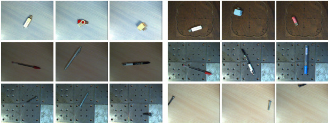
Figure 2: Example images from the robustness validation dataset. Objects in the same row are expected to be clustered in the same group. The five different background/lighting conditions are represented in this figure.
