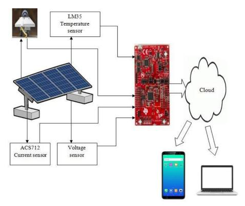
Figure.8 Hardware implementation of proposed work
