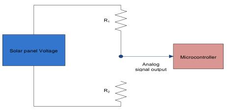
Figure.4 Voltage divider circuit
