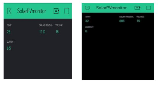
Figure.10 Real-time Solar PV monitoring system using Blynk
