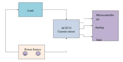
Figure.5 Schematic layout of the current sensor
