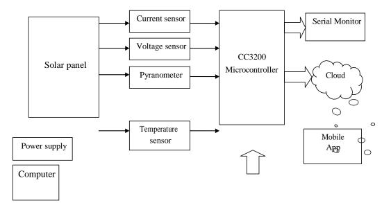
Figure.3 Real-time Solar Energy Monitoring System
