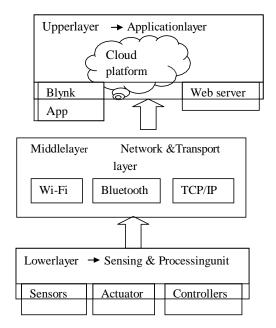
Figure.2 Three-layer architecture of Internet of Things
