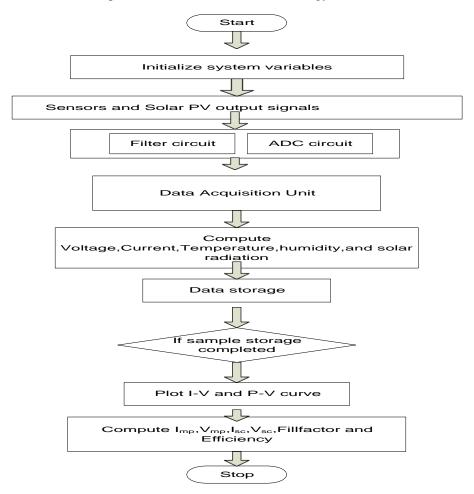
Figure.1 Virtual Solar PV monitoring system using LABVIEW
