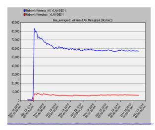
Figure 9. The wireless LAN throughput in the scenario 1 and scenario 2
