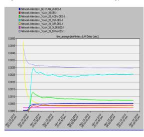
Figure 14. Comparison of Average delay in the wireless network for 40 Nodes
