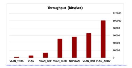
Figure 13. The wireless LAN throughput for 20 Nodes
