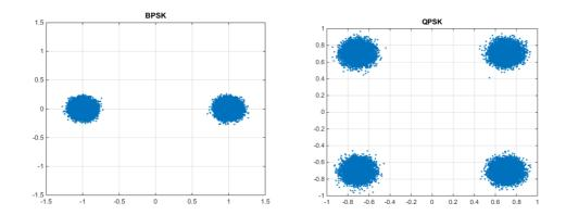
Figure 2: Output constellation of BPSK and QPSK signals
