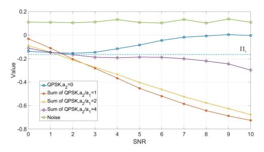
Figure 6: Dependence of cumulants on the SNR for various ratios of the amplitudes of the signals.
