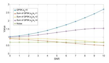
Figure 7: Dependence of normalized constellation radiuses on the SNR for various ratios of the amplitudes of the signals
