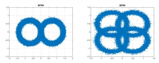
Figure 3: Output constellations for the sum of two BPSK signals and the sum of two QPSK signals with equal amplitudes
